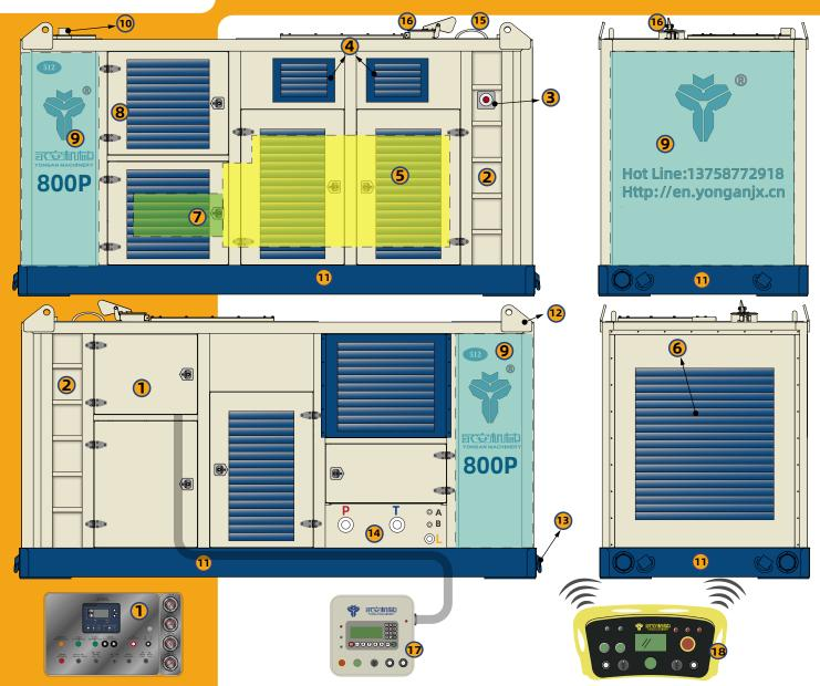
Local control & instrument panel 2. ladder 3.emergency stop switch 4. Engine intake
